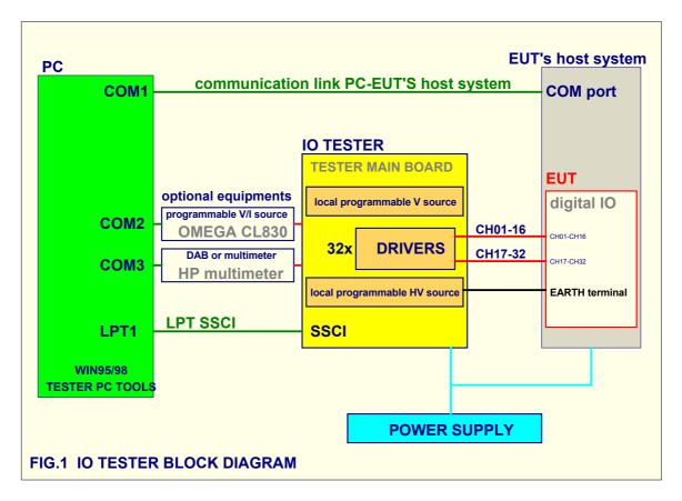
The EUT is tested, calibrated, or serviced in connection with its host system. The EUT's host system must be equipped with a communications port and a software interface enabling the access to data processed by the EUT.
