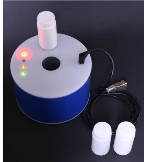
Figure 1. PT01109-1 radiation detector with standardized 100mL sample containers.
